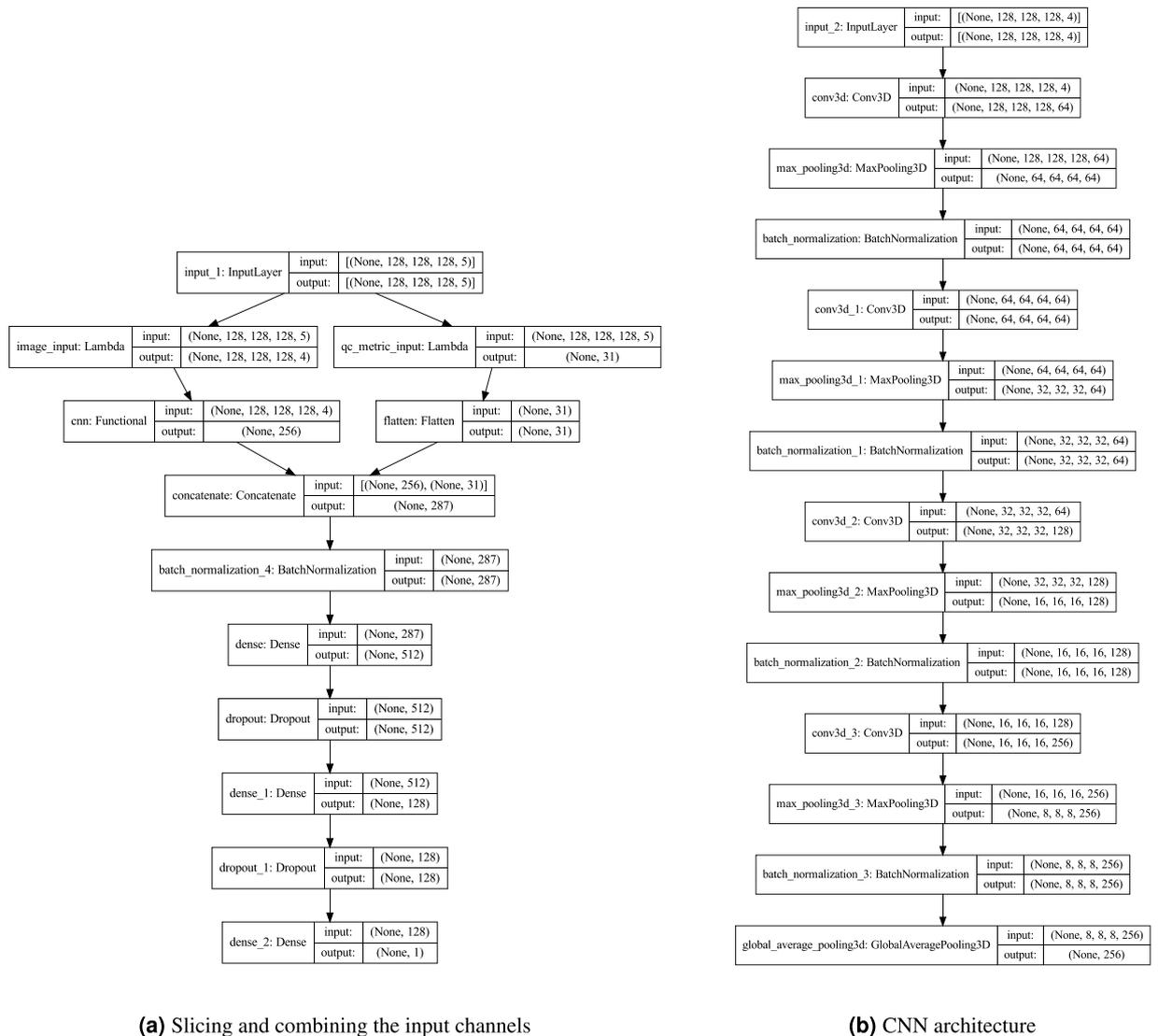
**(a)** Slicing and combining the input channels **(b)** CNN architecture
